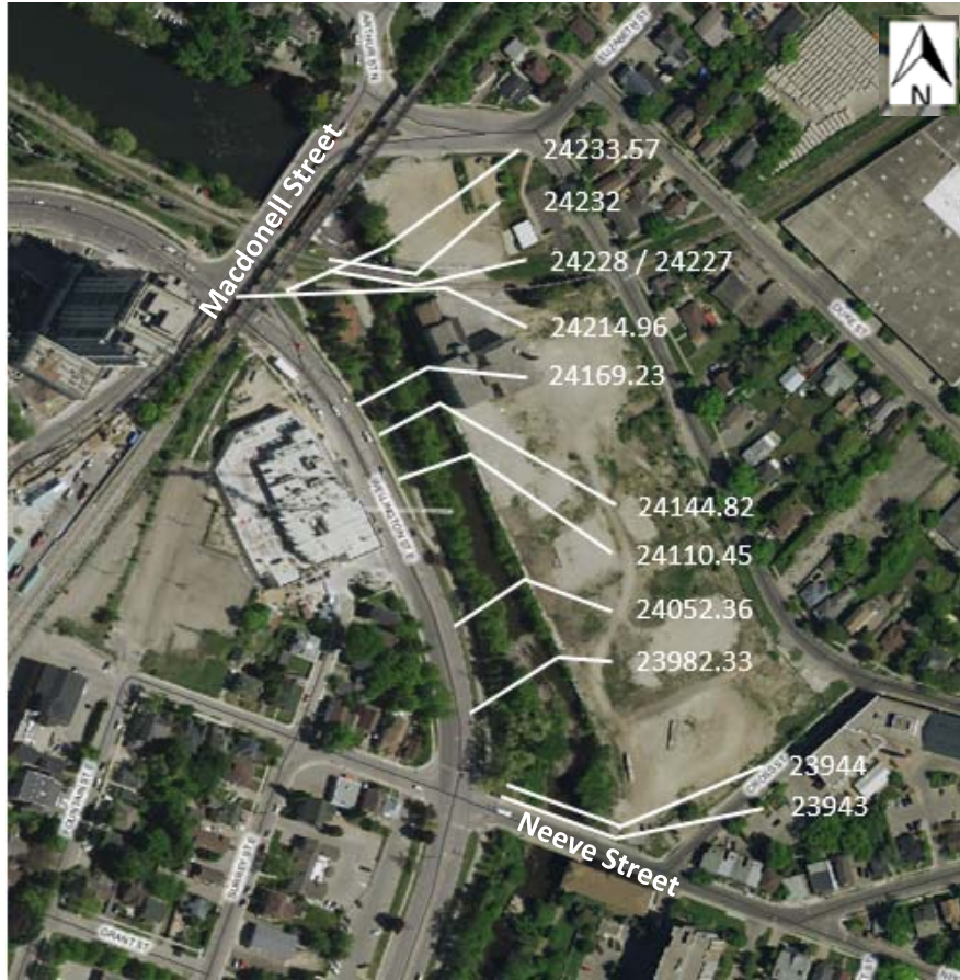
Figure 3-3. Location of HEC-RAS sections (airphoto from Google Maps extracted 2017)
