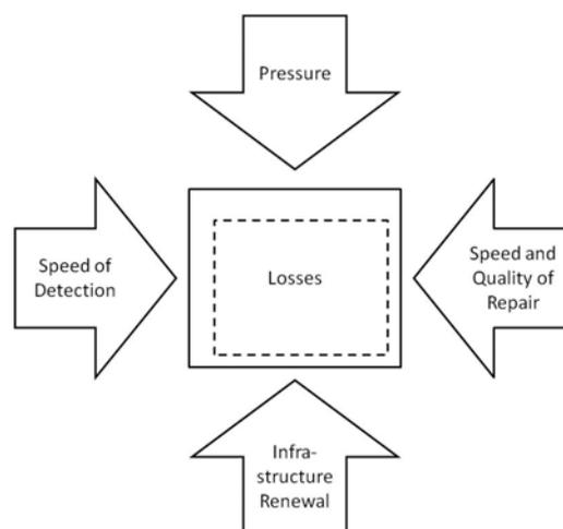
Figure 18 The four influences on leakage (D Pearson)
