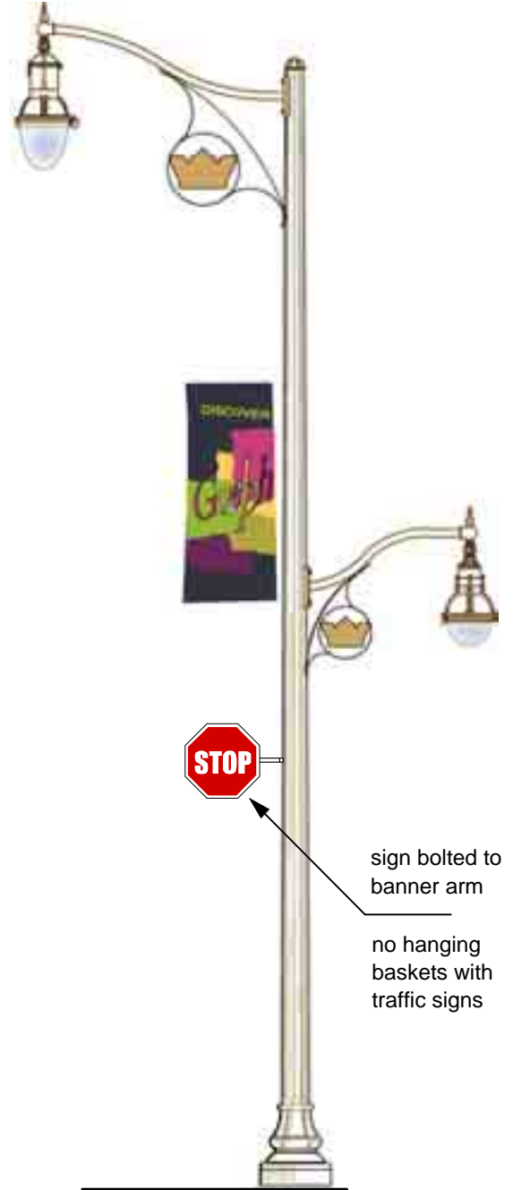
Traffic Sign on Light Pole
